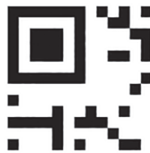
Figure I.3 — Data modules placed in symbol prior to data masking
