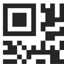
Figure I.4 — Final version M2-L symbol encoding 01234567
